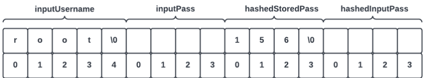
Figure 4: Memory layout after hashing the entered username
