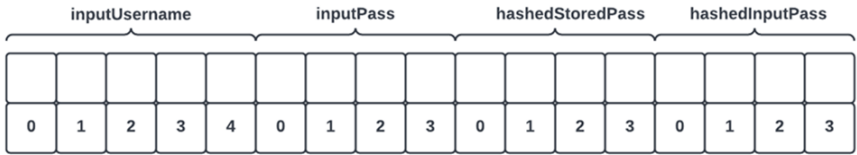
Figure 3: Memory layout after creating variables
