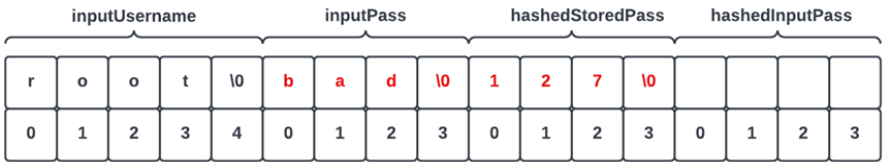
Figure 5: Memory layout after reading the manipulated password
